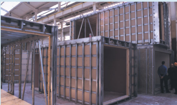
Ayrframe modules in Rollalong's factory
